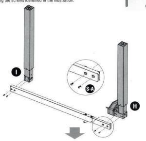
· Tighten all screws with a proper screwdriver.
