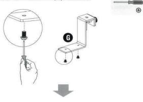
Fix the hooks to the shelf with the previously removed screws.
