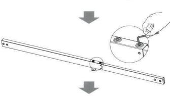
· Attach the telescopic crossbar to the legs as shown using the screws identified in the illustration.
