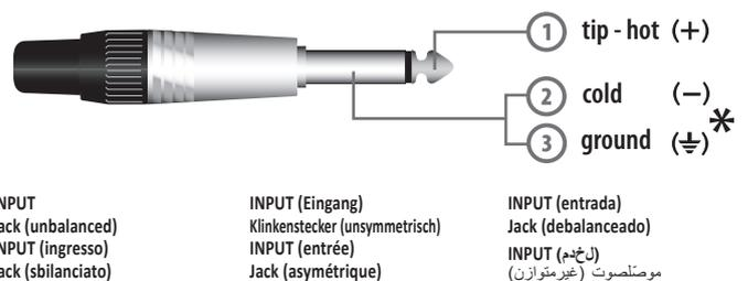
\*note: connect both cold and ground to make cable from balanced to unbalanced
