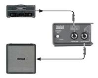
Connect the XLR output to a mic preamp input on your mixing console using a standard XLR microphone cable.
