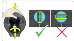
Insert injector from below into opening of machine. Support injector with hand. Rotate injector clockwise until it fits. Follow instructions in "8. DESCALING AT LEAST EVERY 3 – 4 MONTHS" on page 13.
