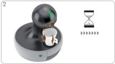
Coffee mix is pressed out of top of capsule holder. Wait until pressing process is finished. This is the case if you hear no noise coming from the machine.
