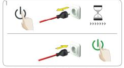
Switch machine off. Check if capsule is blocked, see "9.2 NO LIQUID COMES OUT – CAPSULE / INJECTOR BLOCKED?" on page 15. Unplug power plug and wait 20 minutes. Afterwards plug power plug into mains power socket and switch machine on.
