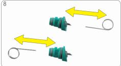
Insert cleaning needle into injector to unclog it. If not possible, prepare a descaling solution with one descaler and 0.5 litre drinking water. Put injector in descaling solution.
