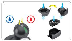
Rinse the machine: Follow instructions in "FIRST USE". Clean with washing-up liquid and fresh drinking water both sides of capsule holder. Rinse drip tray with fresh drinking water and clean it with a clean food-safe brush.
