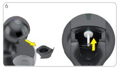
Remove capsule holder. Push injector tool over injector.
