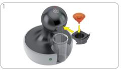
Put rinsing tool into capsule holder. Insert capsule holder into machine.
