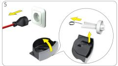
Unplug power plug! Turn drip tray over. Take out the injector tool. Pull cleaning needle out of injector tool. **Keep needle out of reach of children!**
