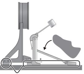
Check to be sure they're making contact with the floor
