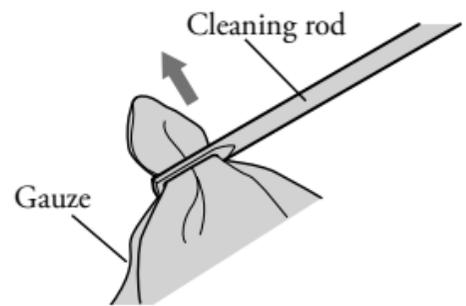
2. Wrap the gauze around the end of the cleaning rod, making sure no bare metal is exposed.
