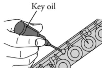
2. After applying oil, move the key several times to spread the oil evenly.
