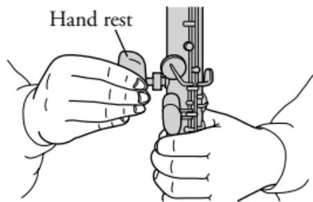
2. Taking care not to press to the keys, hold the body at its uppermost point, and the footjoint by its lowest point, and attach the footjoint to the body.
