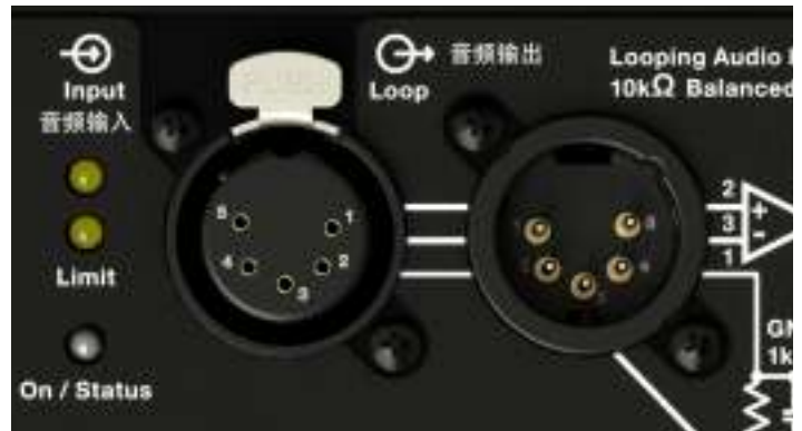
Figure 13: XLR 5-Pin Audio Connectors, Input and Loop Output
