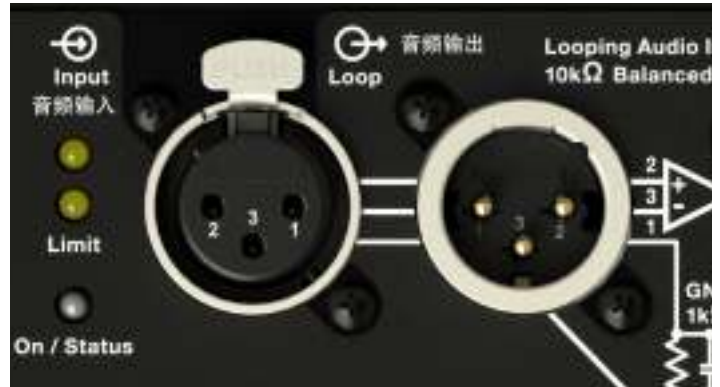
Figure 12: XLR 3-Pin Audio Connectors, Input and Loop Output
