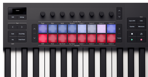
The Launchkey 61 pads reflecting the track select and record arm states on the pads.
